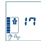
Subsequently, automatic inflation begins. Three short beeps indicate that the necessary inflation pressure has been reached and that measurement is starting.
