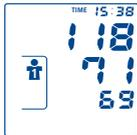
A long beep indicates the end of measurement. Then the systolic and diastolic blood pressure values appear simultaneously one below the other on the display as well as the pulse rate.
